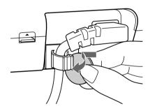
3 Plug the power cord into a grounded AC wall outlet, surge protector, or Universal Power Supply (UPS).
